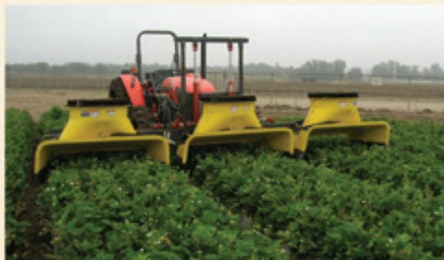
The fans raise and lower hydraulically as well as fold up for transporting. Hydraulic power comes from a PTO mounted pump with a self-contained hydraulic reservoir. PTO HP requirement is approximately 60 HP. We fabricate 3 and 4 row configuration from 48" to 68" beds.
