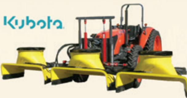
Designed to be **LIGHT** yet **POWERFUL**, the C&N Bug Vac is hydraulically powered with fans that develop 4700 feet per minute suction over the row. This sends all jumping and flying insects into the deflectors like bugs on a windshield.
